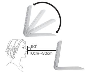
**Adjust for irradiation angle and irradiation distance.**
