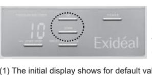
**Please set the timer (maximum for 30 mins) with the UP/DOWN button from the control panel while checking displayed-monitor for irradiation time.**
